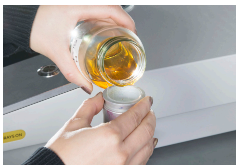
Figure 2: Simply pour the oil sample into the sample cell – no weighing or volumetric measurements required
